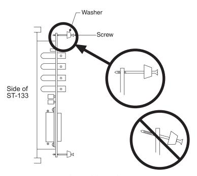
Figure 43. Module Installation
